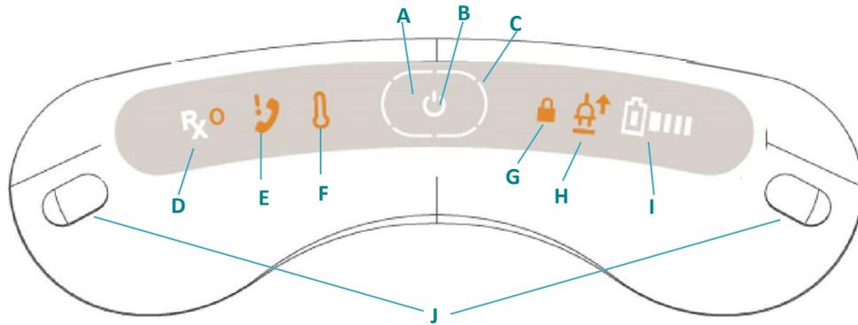
**A. Power Button**
